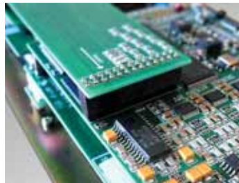
Integrated electronics module which combines powerful Digital Signal Processing with multi-channel class D Amplifiers
